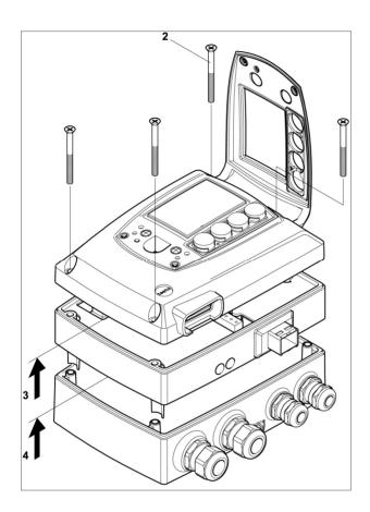
2 Loosen and remove housing screws (2).
