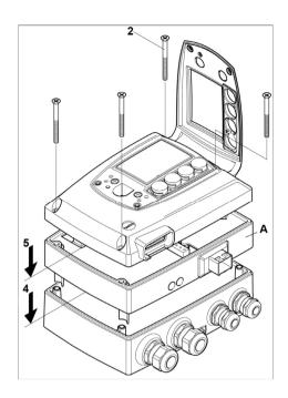
4 Place Ethernet module (A) on lower part of instrument (4).
